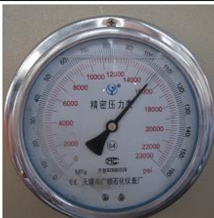
4-1/16"10000psi shell test pressure
