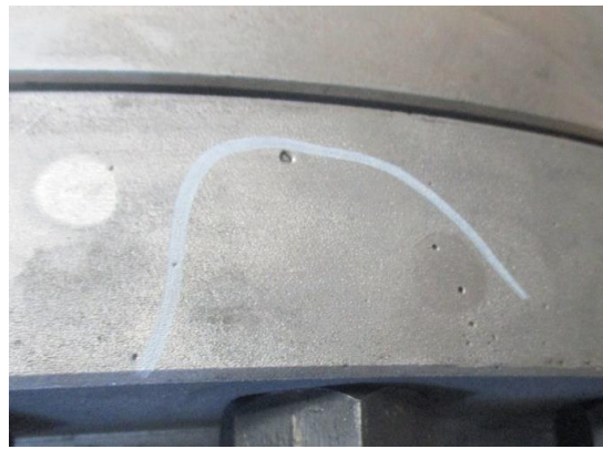
S/N: 9641-001-04 valve casting defects
