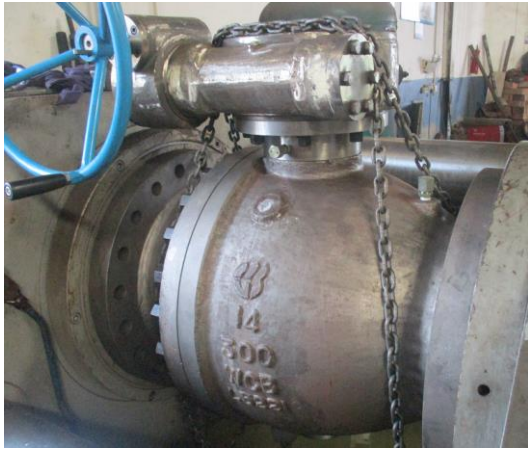
Left Air seat testing
