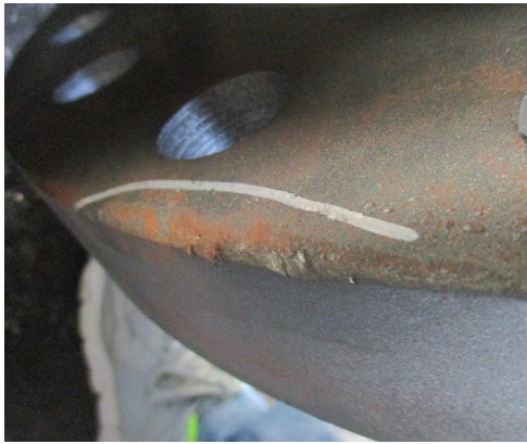
S/N: 9641-001-06 valve casting defects
