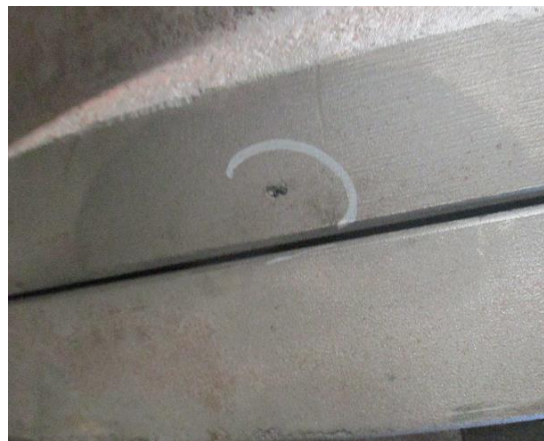
S/N: 9641-001-05 valve casting defects
