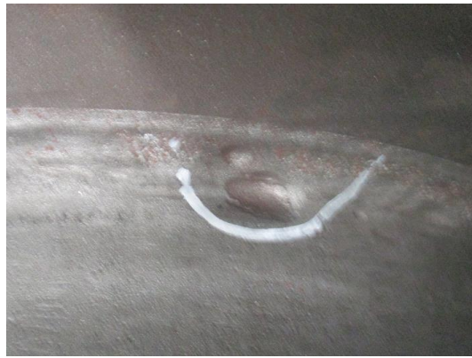
S/N: 9641-001-12 valve casting defects
