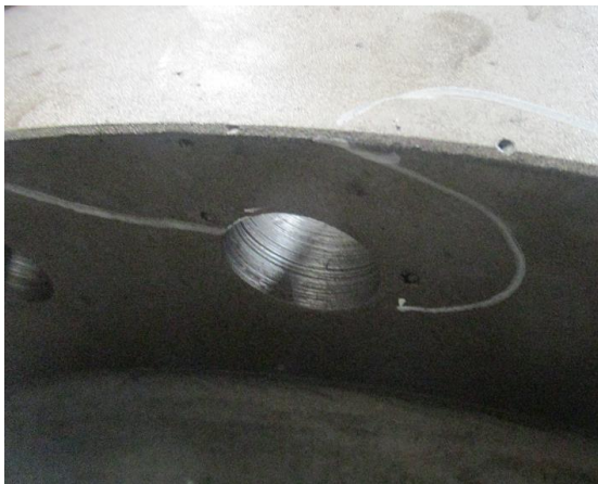
S/N: 9641-001-11 valve casting defects
