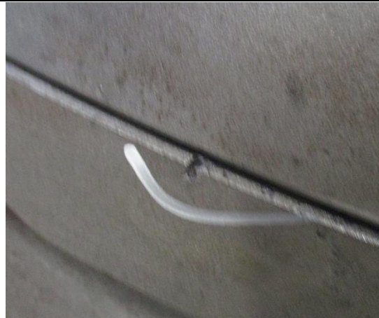
S/N: 9641-001-11 valve casting defects
