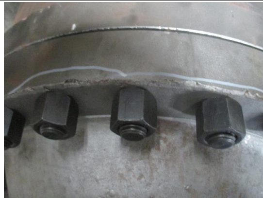
S/N: 9641-001-01 valve casting defects
