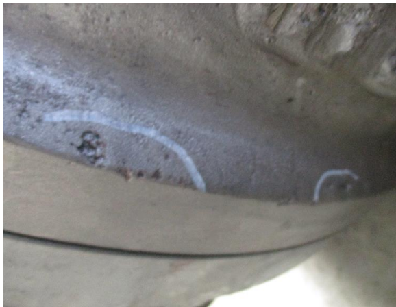
S/N: 9641-001-02 valve casting defects
