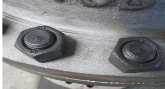
Bonnet marking and stud/nut marking
