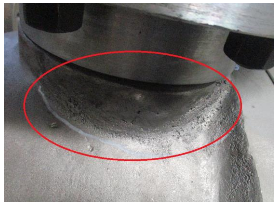
S/N: 9641-001-03 valve casting defects
