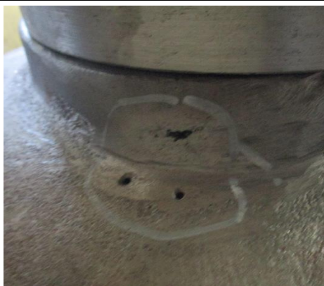
S/N: 9641-001-01 valve casting defects
