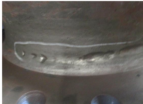
S/N: 9641-001-04 valve casting defects
