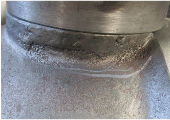
S/N: 9641-001-07 valve casting defects
