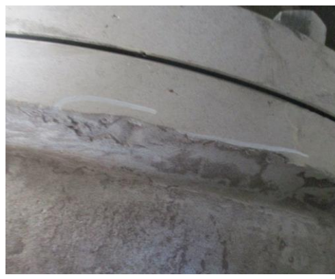
S/N: 9641-001-09 valve casting defects
