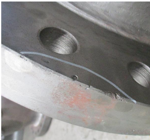
S/N: 9641-001-07 valve casting defects
