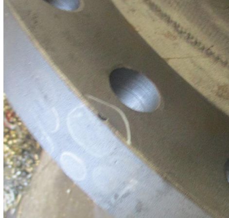
S/N: 9641-001-06 valve casting defects
