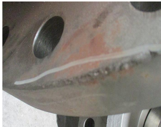
S/N: 9641-001-08 valve casting defects
