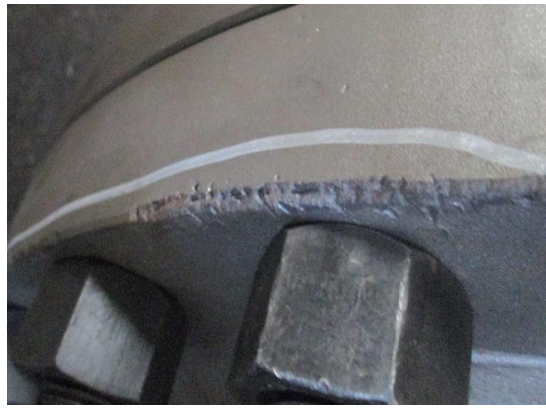
S/N: 9641-001-06 valve casting defects
