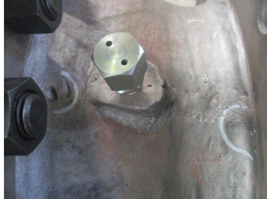
S/N: 9641-001-12 valve casting defects
