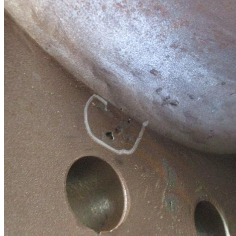
S/N: 9641-001-07 valve casting defects
