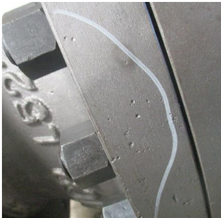
S/N: 9641-001-06 valve casting defects
