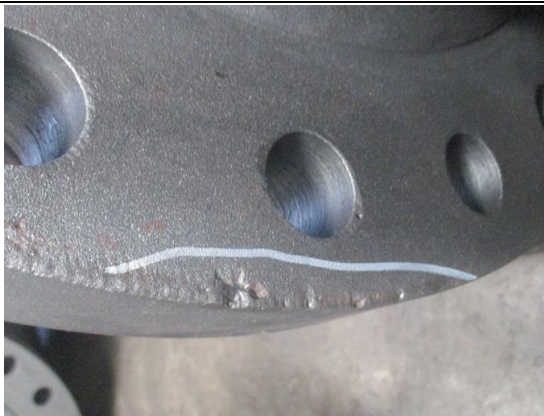
S/N: 9641-001-03 valve casting defects
