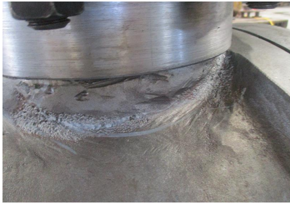
S/N: 9641-001-09 valve casting defects
