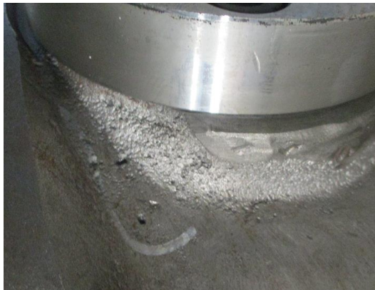
S/N: 9641-001-09 valve casting defects
