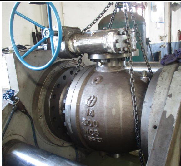
Left Hydraulic seat testing
