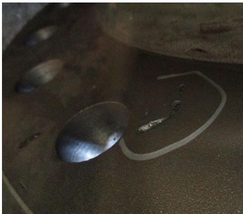
S/N: 9641-001-05 valve casting defects
