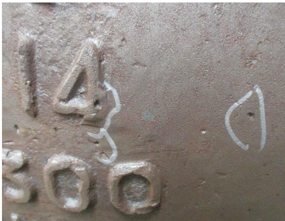
S/N: 9641-001-08 valve casting defects
