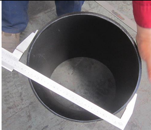
90° elbow 18" STD, the marking hadn't finished, because factory didn't receive the additional marking for this size
