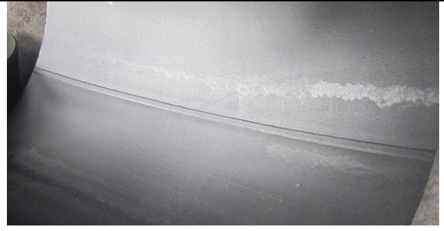
ELBOW 45° L/R 36" SCH STD welding line
