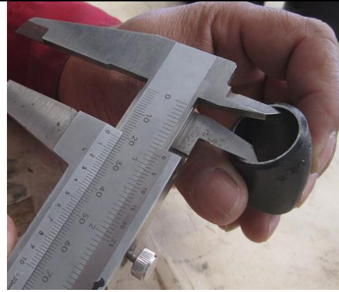
90° elbow 18" sch40, BW end plane requires 1.6 \pm 0.8 mm, but actual dimension is 3.3mm
