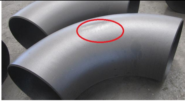
90° elbow 18" STD, the marking hadn't finished, because factory didn't receive the additional marking for this size
