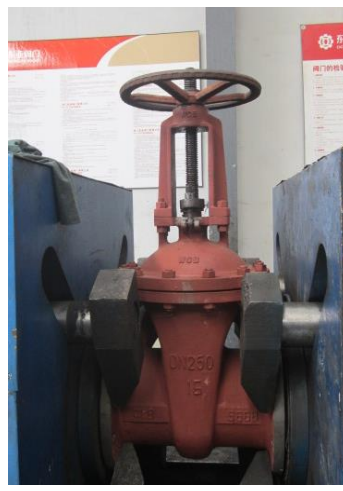
Item28 valve testing
