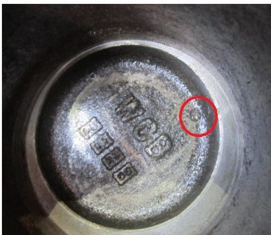
Item12,S/N:15101939, disc casting leakage
