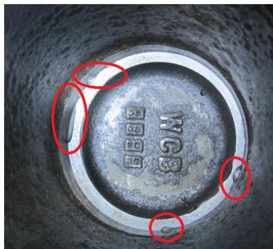
Item12,s/n:15101957,hydraulic seat leakage
