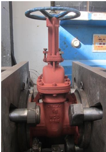
Item21 valve testing
