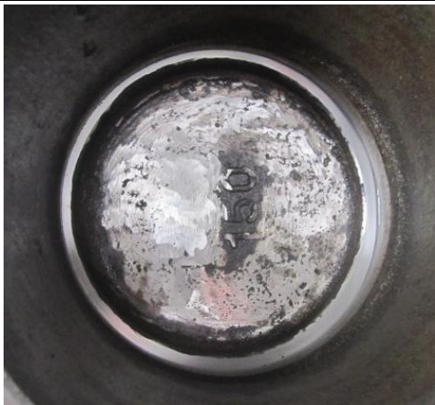
Item17, s/n:15102011/15102022, the disc surface roughness isn't good
