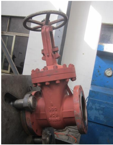
Item48 valve testing
