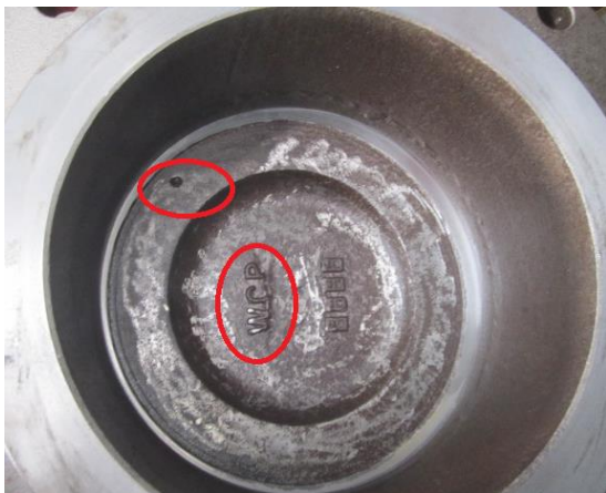
Item16, the bore and disc are rusty, the disc has air hole, the "WCB" marking isn't clear
