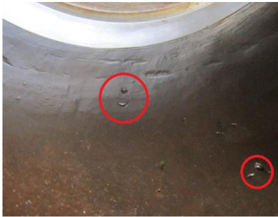
Item28, the bore and disc rusty, bore has defects
