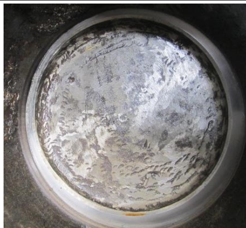
Item21/22, the disc surface roughness isn't good
