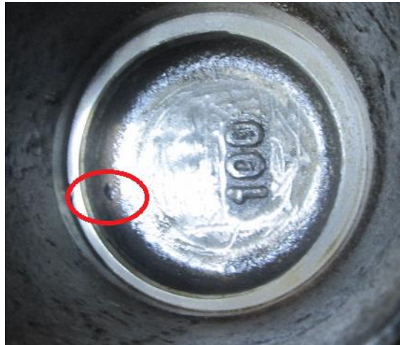
Item12, s/n:15101957, the disc has air hole
