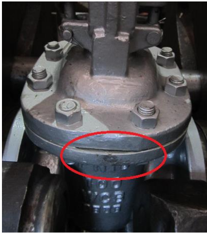
Item12, s/n:15101939, the body and bonnet flange misalign
