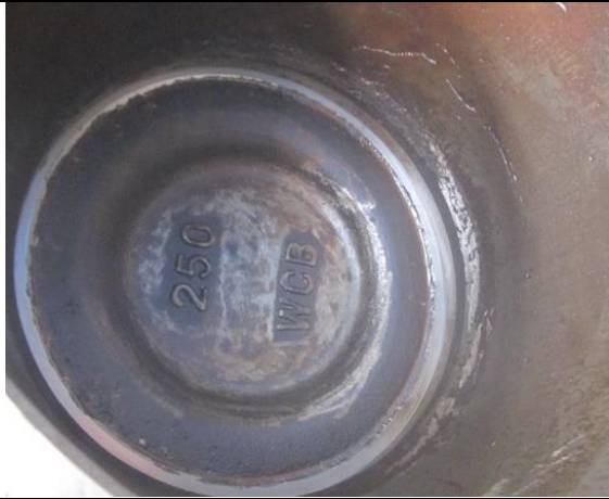
Item28, the bore and disc rusty, bore has defects
