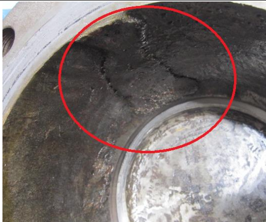
Item 21, the bore has sand inclusion
