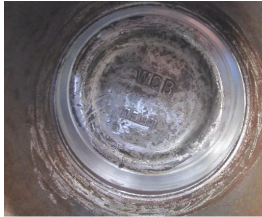
Item30, s/n:15102701, the disc surface roughness isn't good
