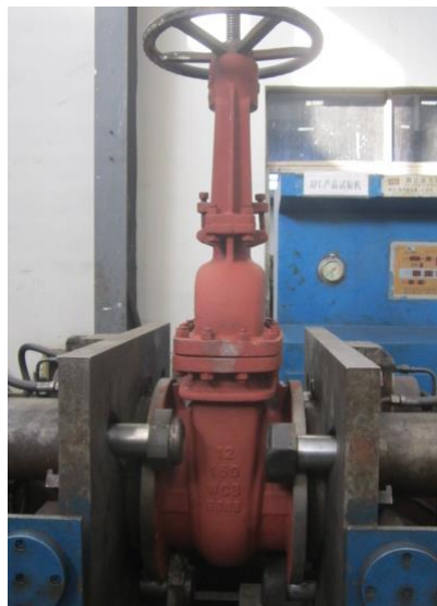
Item 16 valve testing
