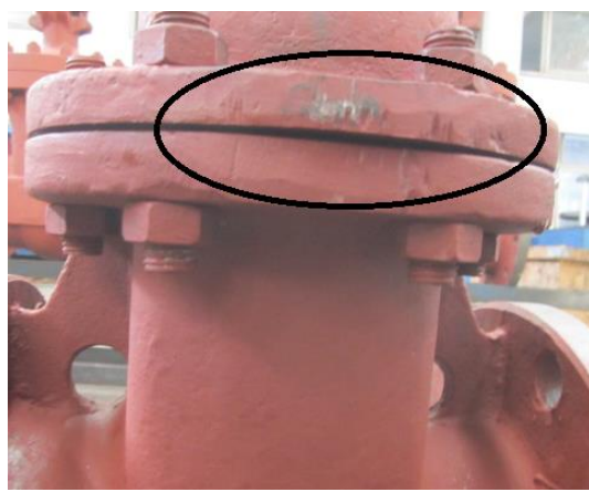
Item17, s/n:15102009, the body and bonnet flange misalign
